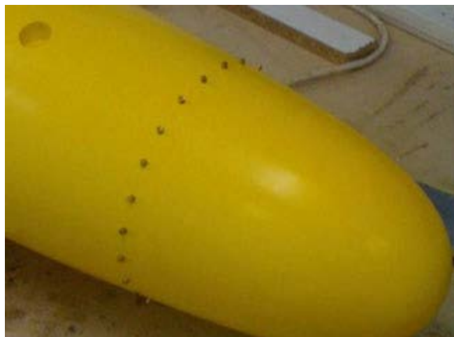
(e) Trip studs on towing tank model (courtesy of AMC)
