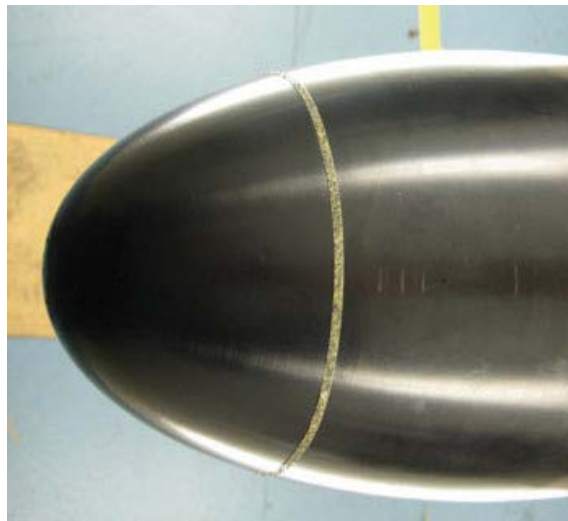
(b) Grit on wind tunnel model (courtesy of DST Group)
