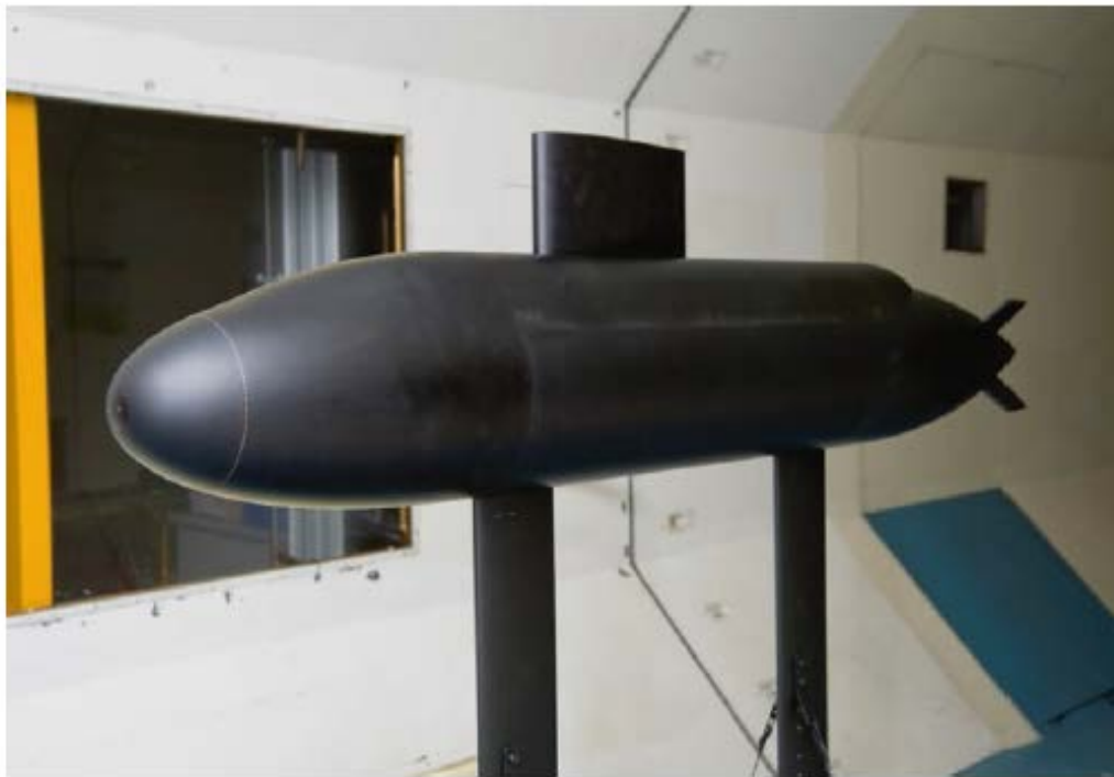
Fig. 4.14 Submarine model being tested for resistance in a wind tunnel (courtesy of DSTO)
