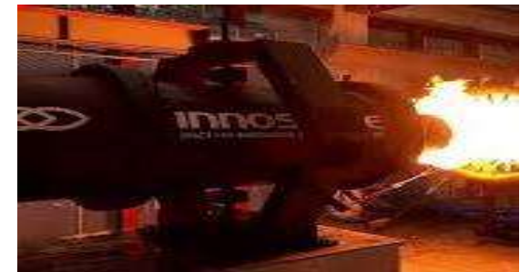
Innospace: Hyper-15 Hybrid Rocket Paraffin/LOX Propellants ISP ≅ RP-1/LOX Thrust: 150KN
