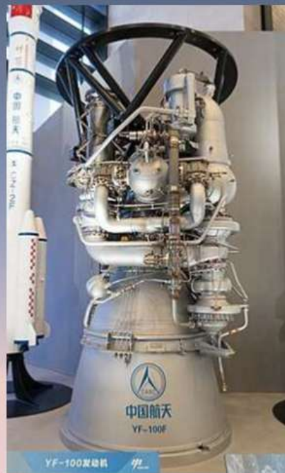
Model: YF-100 Propellants: RP-1/LOX Thrust: 1340kN @ vacuum Chamber Pressure: 180 bar ISP: 335 sec @ vacuum Application: LM5~LM8
