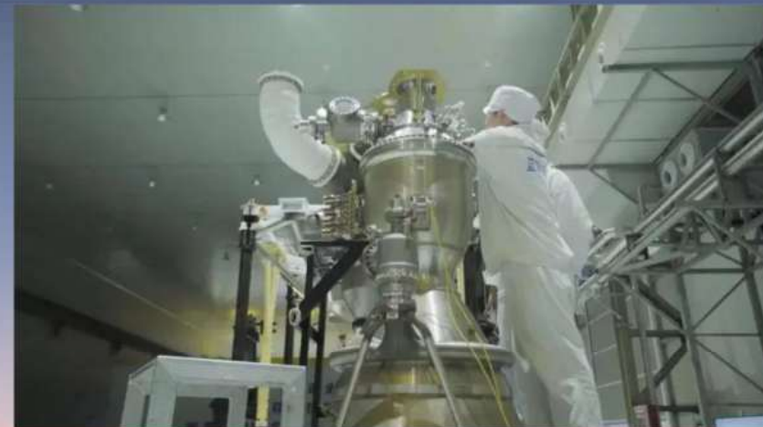
Model: TQ-12(天鵝) Propellants: CH4/LOX Thrust: 785kN @ vacuum Chamber Pressure: 101 bar ISP: 337 sec @ vacuum First hot fire: May 2019 Application: ZQ-2(朱雀二號) Manufacturer: LandSpace
