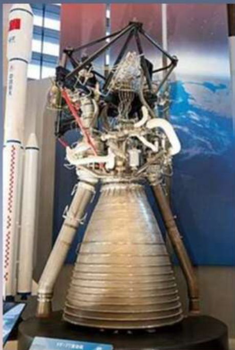
Model: YF-77 Propellants: LH2/LOX Thrust: 700kN @ vacuum Chamber Pressure: 101 bar ISP: 428 sec @ vacuum Application: LM5
